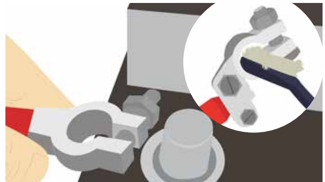
Figure 20 - Nettoyage des batteries
