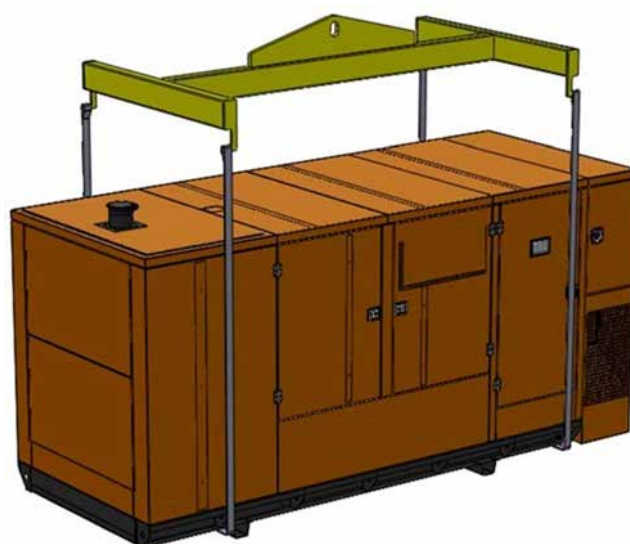
Figure 11 - Elevation with lifting straps. Soundproofed genset.
