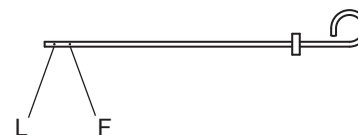
Oil level check (4Y / 1DZ Engine)
