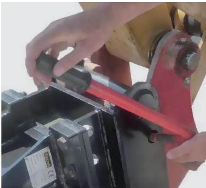
FIGURE 20: Releasing the hydraulic breaker
