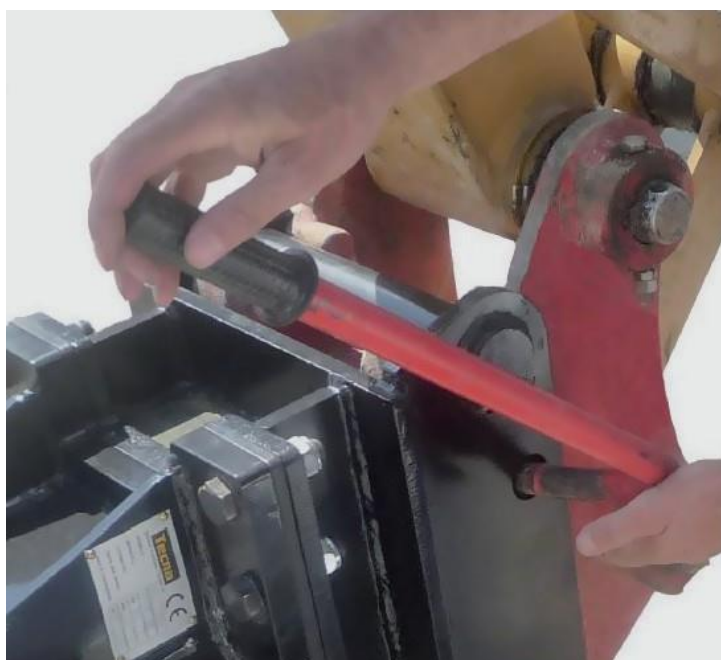
FIGURE 5: Securing the hydraulic breaker
