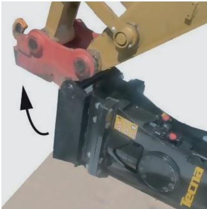
FIGURE 21: Removing the connection to the quick-changer (step 1)
