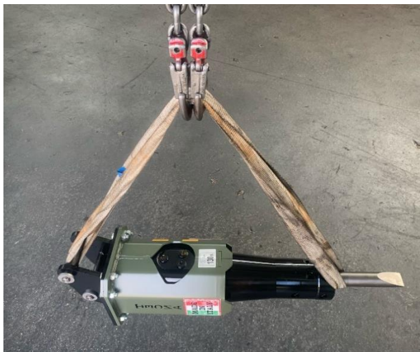
FIGURE 3 – Position of the lifting strap
