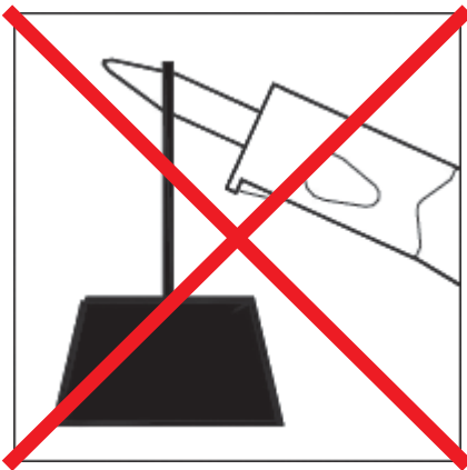
FIGURE 18: Hydraulic breaker is not a lifting tool
