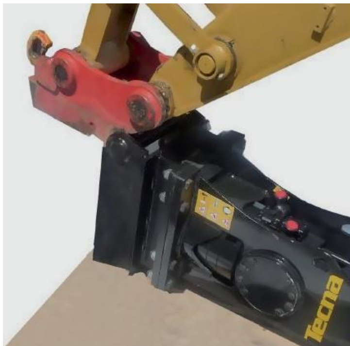
FIGURE 4: Holding the hydraulic breaker
