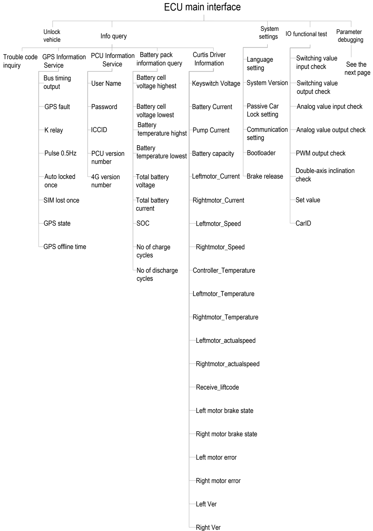
Figure 6-18 System interface description
