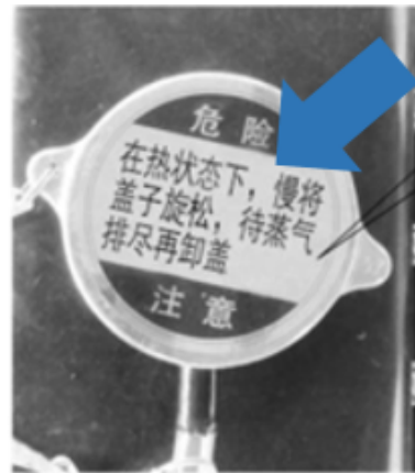
Fig. 17 Pressure cap on the radiator
