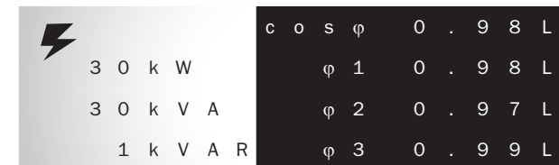
Fig.2 cosφ: Total power factor / φ1: Power factor phase 1 φ2: Power factor phase 2 φ3: Power factor phase 3
